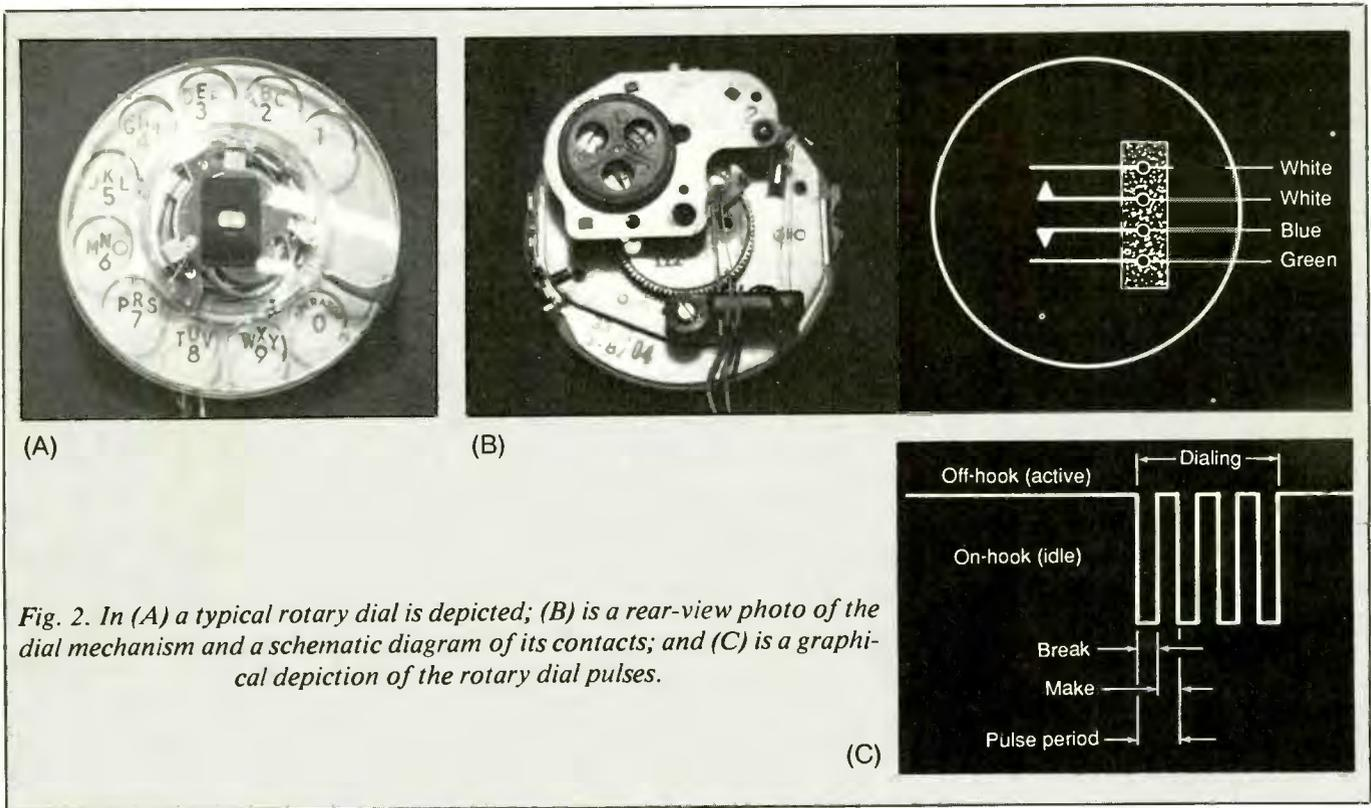
Fig. 2. In (A) a typical rotary dial is depicted; (B) is a rear-view photo of the dial mechanism and a schematic diagram of its contacts; and (C) is a graphical depiction of the rotary dial pulses.
