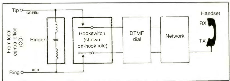
Fig. 6. Simplified diagram of a conventional single-line telephone.
