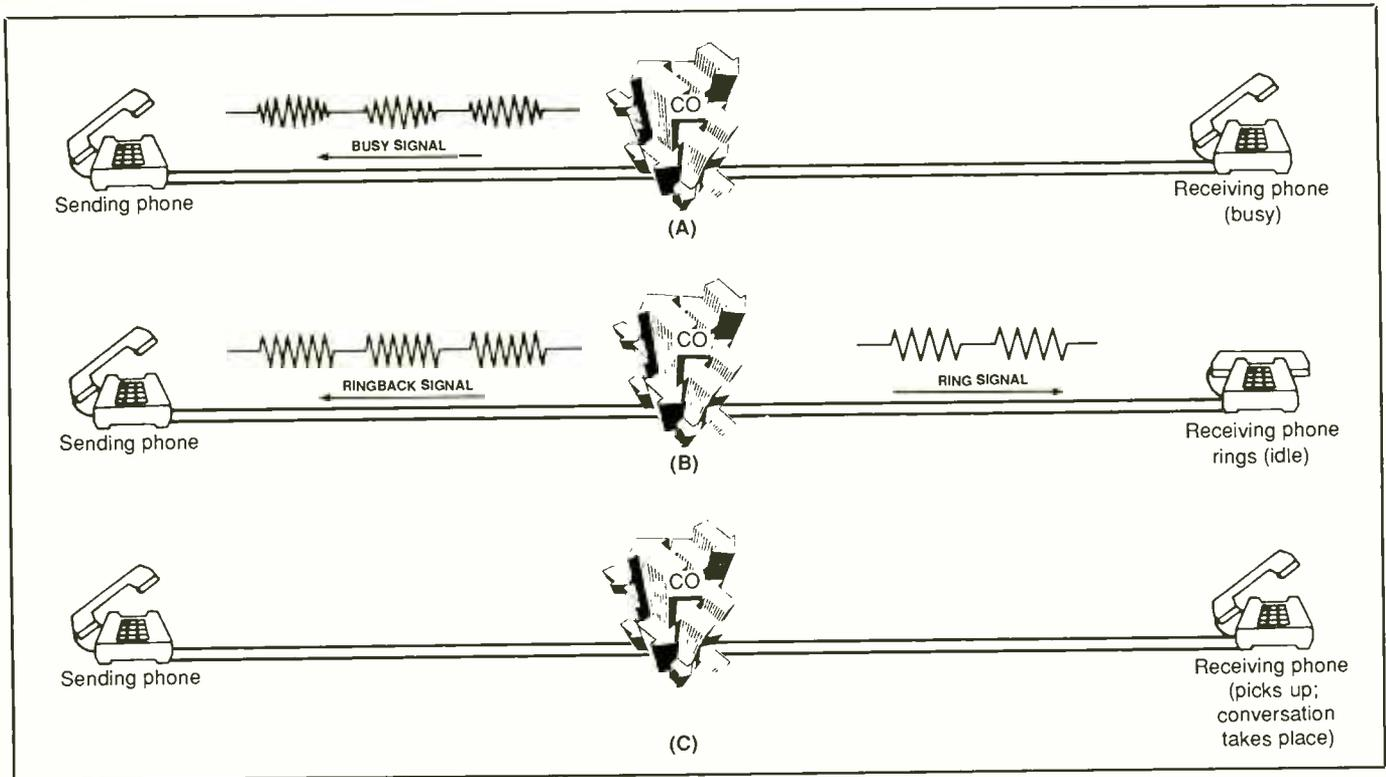
Fig. 9. Central Office returns to an originating instrument a busy signal or a ringback signal when the phone being called is (A) off-hook or (B) on-hook. It makes a through connection (C) when the receiver of the instrument being called is picked up.
